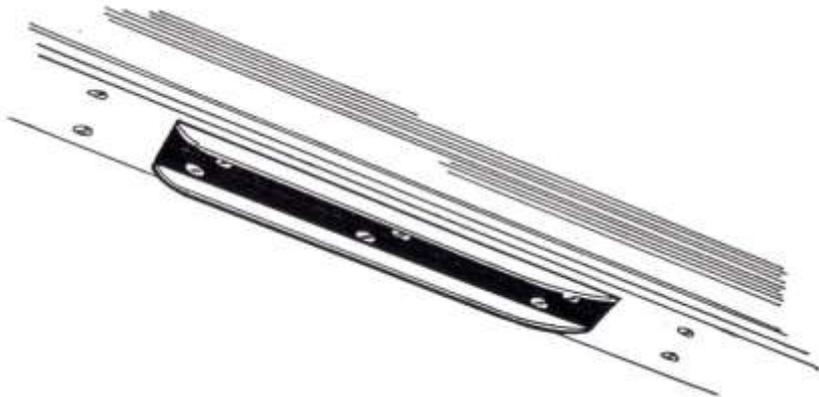
These sharp steel non-skid shoes are used to stop the PolyPod SnowCamper Sledge from side-slipping when traversing glacial slopes.
